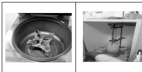
Figure 2 Washing of A. hydrophila isolate by centrifugation Degradation of cell walls of A. hydrophila using sonication
